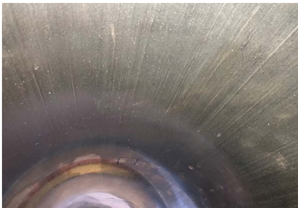
Fig. 1 Cylinder liner scuffing
